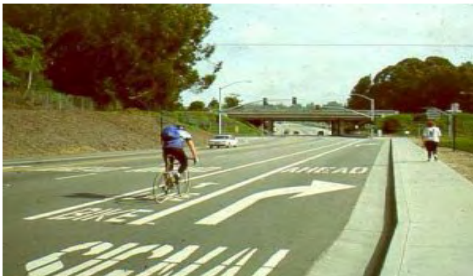
Example - Bike lane with roadway signage
